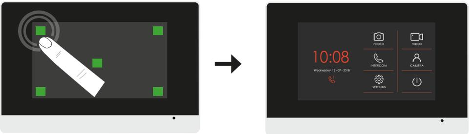
On start up, press on the 5 green targets which appear one after the other in the four corners of the screen and in the center. Wait until the main screen appears.
