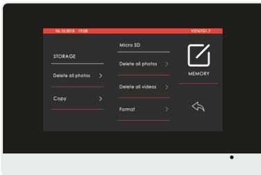
Copy : copy the photos from the monitor to the micro SD card in the BKUP PIC folder.
