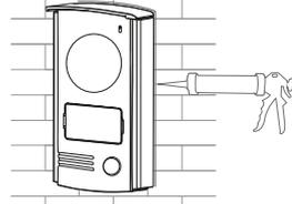
After installing and test, place a transparent acid free silicone seal at the top and on the sides of the door station (not at the bottom) to avoid any risk of infiltration.
