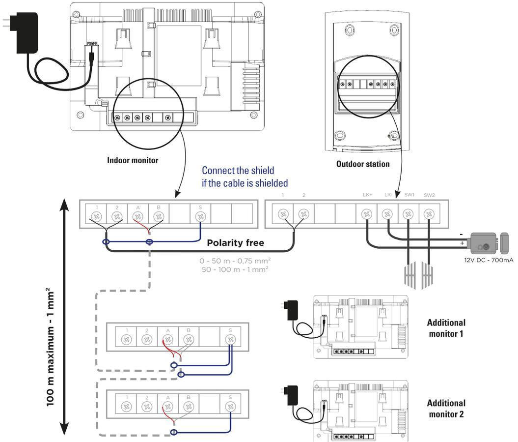
Until two additional monitors for a total limit of distance of 100 m
